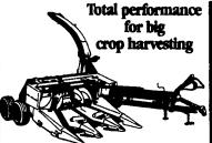
You get total performance when you harvest your crops with a Model 900 forage harvester. Total performance begins at the cutterhead. The 12 knives of the 21-inch cutterhead give you uniformly cut, high-quality forage. Other leatures on the "900" include:
