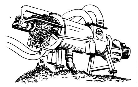
Agway now has the slurry separator to meet your needs. This unit produces solids that will compost and liquids that will irrigate or inject.
