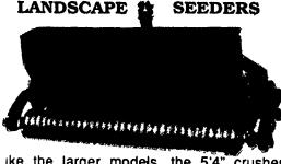
Like the larger models, the 5'4" crushes, seeds and rolls in one operation, tucking seeds in the top 1/4" of the soil... in a firmed clod-free seedbed that gives thick, even stands at greatly reduced seeding costs. The shallower seeding depth is just right for controlled moisture and growth conditions.
