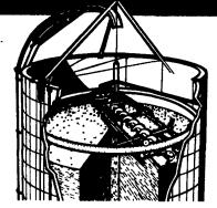
The Jamesway Big Jim system unloads silage from the top, then discharges it down a big preformed center hole and out the bottom. Result: You can store high moisture silage — with more total feed value than low moisture silage — without cold weather worries. And without the big price tag of oxygen-limiting, bottom-unloading systems. See us soon for details.
