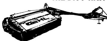
Gehl has two all-new disc mower conditioners to cut your crop down to size, fast and easy. The DC2340 has 7 discs and a 9-foot cutting width; the DC2360 has 8 discs and a 101/2 -foot cutting width.
