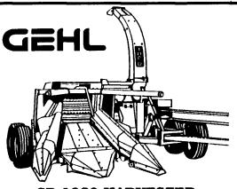
**CB 1060 HARVESTER** 1 Only #7312 1000 RPM, Elec. Controls, Less Corn Or Havhead, Single Axle With 12.5Lx15 Tires
