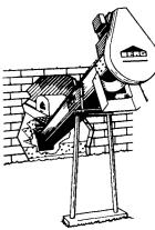
...with a BERG AUGER MANURE CONVEYOR! Installed at the discharge end of your barn cleaner or at any inconvenient mid-point, the continuous, spiraling action of the big 12" revolving auger
