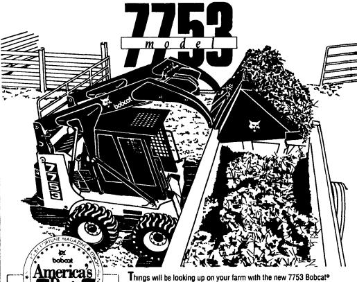
Skid-Steer loader It's the ideal lift and carry machine, with a rated operating capacity of 1700 pounds to lift those big loads higher and further. And, with its push-button auxiliary controls built into the steering lever, you have finger tip control of your attachment 7753 Features:
