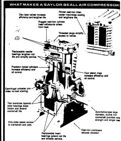
ALL COMPRESSORS ARE AVAILABLE WITH EITHER SPLASH LUBRICATION OR PRESSURE LUBRICATION
