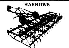
CART MOUNTED HARROWS. Allows each section of the harrow to follow the contour of the ground but also has a cart that converts the machine for easy trans-
