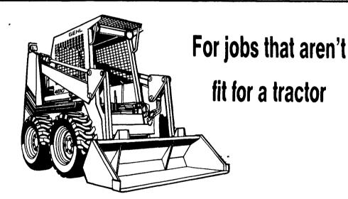
The Gehl 4510/4610 Skid Loaders are the machines you can count on to get the job done. The more you use a Gehl Skid Loader, the better you'll like the job-tough, time saving features: • Self-leveling lift action • Side mounted Load-Trak T-bar controls • Easy to view instrumentation • Roll-back ROPS for easy serviceability • High-output hydraulics for smooth operation of a wide range of attachments • And much more. See
