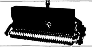
With its 3-point hitch (Cat. I), the Brillion 5'4" Landscape Seeder close-couples to your tractor; works up close to buildings, fences and sidewalks. Seeding mechanism stops instantly when seeder is " of soil for best germination under controlled moisture. Seeding rate is approximately four times that of Turfmaker.
