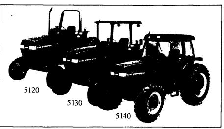
CHOOSE FROM 3 MODELS 5120 — 77 PTO hp, 16F/12R SYNCHROMESH OR 16F/12R POWERSHIFT TRANSMISSION 5130 — 86 PTO hp 5140 — 94 PTO hp
