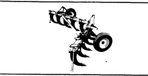
SUBSOILER, A POPULAR, VERSATILE SOIL MANAGEMENT TOOL designed with husky. curved shanks, the subsoller digs down as deep as 16". It opens up the soil allowing moisture to penetrate, roof systems are no longer restricted and better drainage results. Available in 3-11 Shanks.
