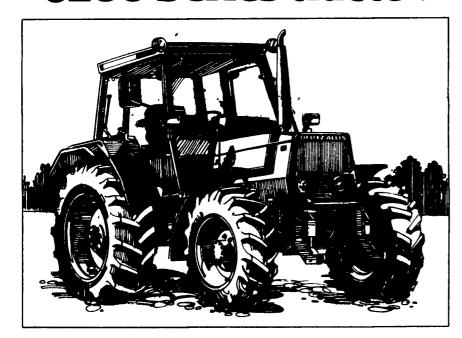
Sized and priced just right for a variety of farm work, Deutz-Allis 6200 Series tractors bring you the economy of Deutz aircooled diesel power. Choose from 43 to 71 hp, with 2-wheel or all-wheel drive and available cab. You'll have a durable Deutz AirDiesel engine and your choice of optional features, such as PTO and 3-point hitch at both front and rear.
