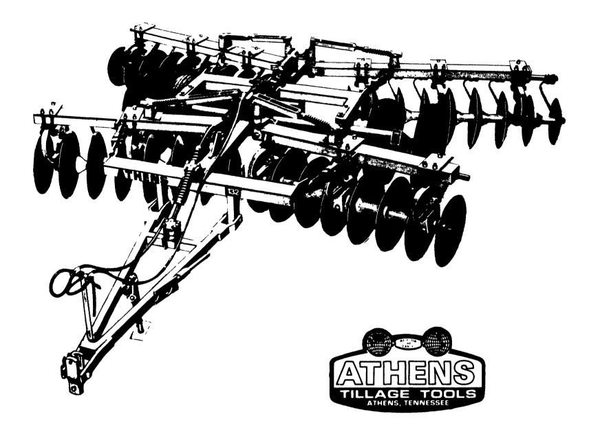
Athens Plow Company, Athens, Tennessee will manufacture the Model 132 Flex Harrow in limited production for 1991. The Model 132 combines the best features of their popular Model 131 with the addition of spring bearing hangers and double tapered Timken gang bearings.
