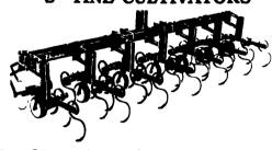
The "S" tine has a four-way tooth movement that is designed for high speed cultivation in conjunction with chemical weed control The spring tines perform well in dry or wet soil, even in rocky ground. The vibrating tines not only kill weeds, but also mulch the soil and level the ground. 4, 6, 8 & 12 row.
