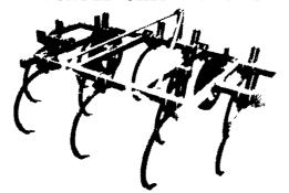
The CPP series of mounted models enables you to turn short and fast... to transport easily, utilizing your tractor's hydraulic system. 7, 9, 11, 13 or 10, 12, 14, 16 ft.
