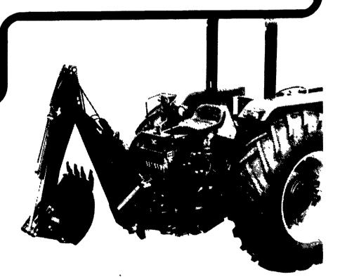
3-point hitch available for all models with universal weight transfer assembly that provides rigid tractor mounting of backhoe for efficient digging per-
