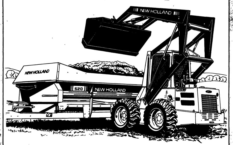
New Holland L-550 Series skidsteer loaders handle loads with greater efficiency. Model L-550 loaders are highly maneuverable, and can lift up to 1,700 pounds (SAE). Their longer wheelbase lends greater stability and the exclusive boom lift linkage lets
