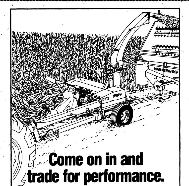
When it comes to harvesting, you can't beat the heavy-duty performance that's built into the New Holland Model 790 forage harvester. Performance starts at the cutterhead. The 19<sup>11</sup>/<sub>16</sub>-inch wide, 12-knife cutterhead delivers a fine uniform chop that's just right for most silage feeding operations. And an electric clutch gives instant response and positive control on the reversing gearbox. The Model 790 is available with either a 540 rpm or 1000 rpm PTO drive.
