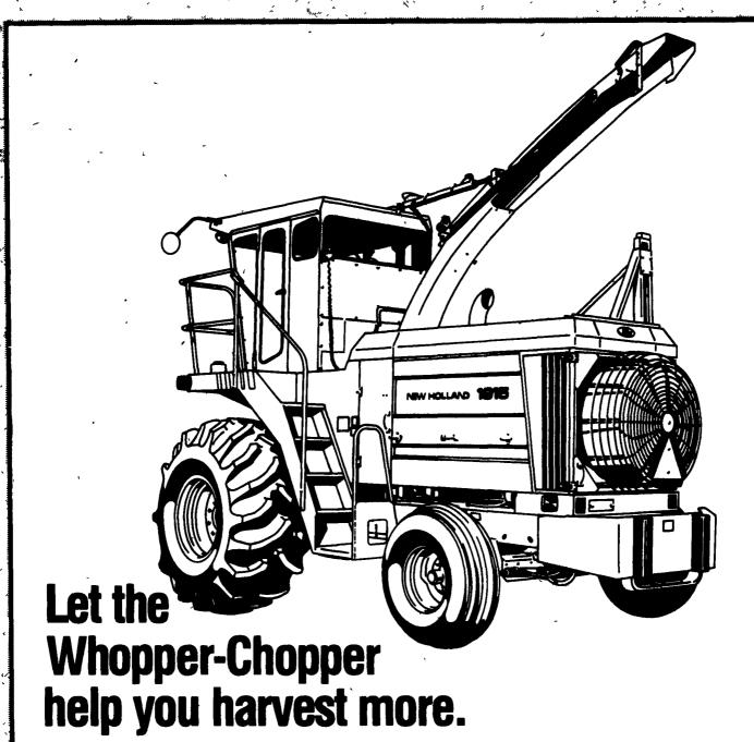
If you custom harvest as well as chop your own forage, the self-propelled Whopper-Chopper Model 1915 can help you harvest more crop at peak quality. The fuel-efficient 270-horsepower diesel engine and the 24-inch, 12-knife cutterhead give you high capacity day-in and day-out harvesting. And an interchangeable crophead system features a one-auger base feed system that lets you mount either a four- or five-row cornhead or a Super-Sweep windrow pickup.
