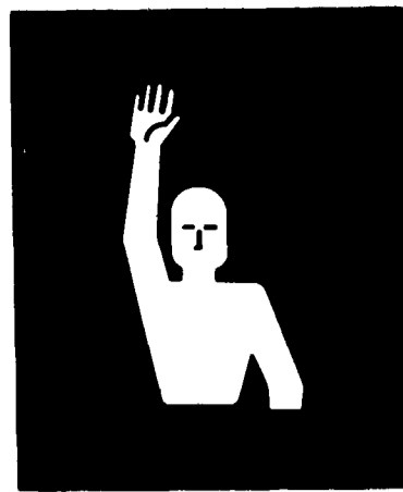
STOP —Raise hand upward to the full extent of the arm, palm to the front. Hold signal until understood.
