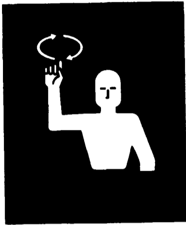
RAISE EQUIPMENT —Make a circular motion with either hand at head level.
