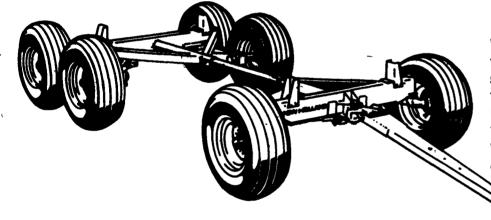
Whether you need a wagon for light- or heavy-duty hauling, there's a farm wagon from Ford New Holland that's the right size for you. Three models have ASAE load ratings ranging from 8½ tons to 12½ tons. The Model 612 (shown above) is designed to take the stress of heavy-duty forage boxes that need maximum flotation. It's the biggest and strongest wagon ever offered by Ford New Holland. Stop in soon and ask about it.
