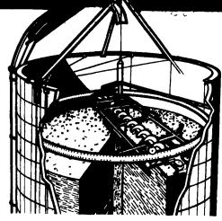
The Jamesway Big Jim system unloads silage from the top, then discharges it down a big preformed center hole and out the bottom. Result: You can store high moisture silage—with more total feed value than low moisture silage—without cold weather worries. And without the big price tag of oxygen-limiting, bottom-unloading systems. See us soon for details.
