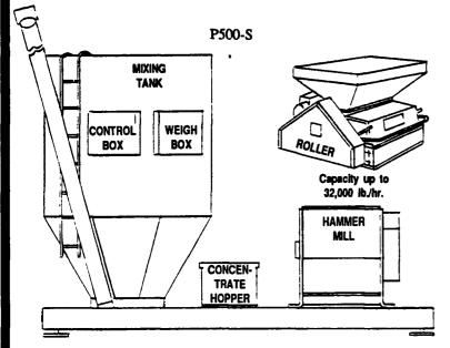
Options: 10" dia. x 10" long rolls (hard chrome surface) including hopper, iron trap, guards, discharge stand with motor mount, 5 ft. x 5.5 ft. belt drive auger for discharge ..........\$3,320.00 Micro processor for batching Freight not included. Price is firm for 30 days.
