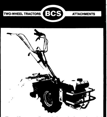
The world's most versatile two-wheel tractor has become the standard of the industry for rear tine tillers. With heat-treated all gear drive, 100% ball bearing construction (no bushings), low profile, the best "power to weight ratio" offered, plus standard safety features and unmatched performance, BCS tractors leave competition in the dust.
