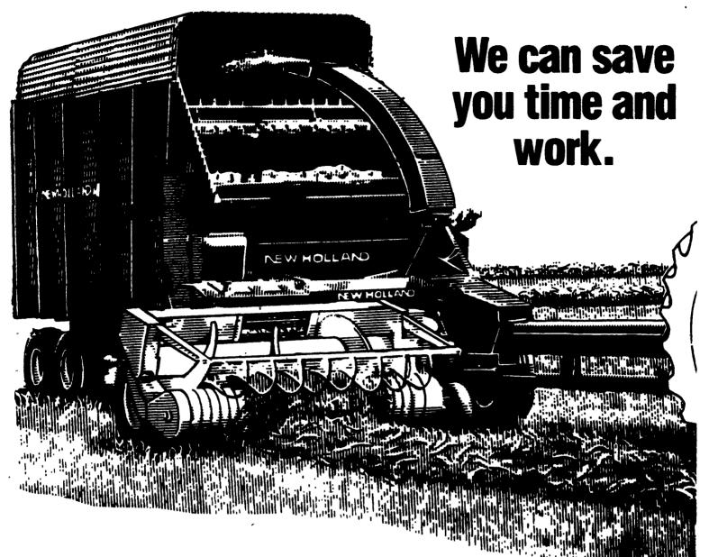
You get total performance when you harvest your crops with a Model 900 forage harvester. Total performance begins at the cutterhead. The 12 knives of the 21-inch cutterhead give you uniformly cut high-quality forage. Other features on the 900 include:
