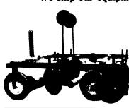
Standard Features • Heavy-duty bolted frame • 2 rollers - one for ground leveling, one to hold plastic down • Depth control wheels • Dirt guards for high-speed laying • Lays mulch plastic - from 3' to 6' wide, fully adjustable • Economy Models as low as 595.00
