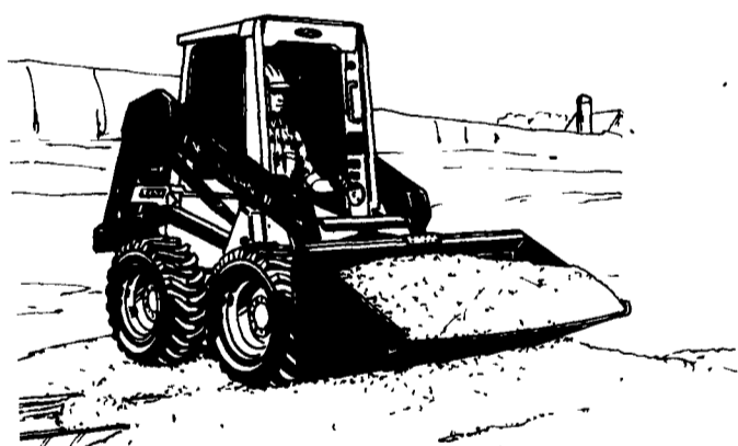
400 SERIES OPERATING LOAD UP TO 1,200#
