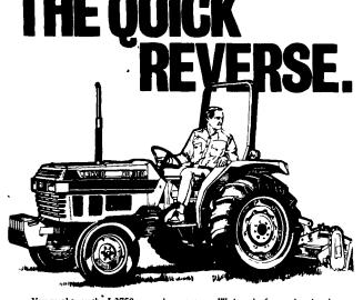
You might say the L3750 is quick on its tires. With eight forward and eight reverse speeds plus your choice of a mechanical or hydraulic shuttle-shift, all kinds of front loader jobs go quick
