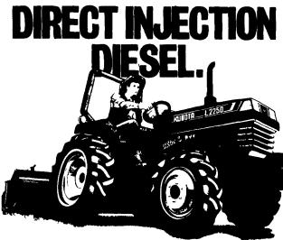
Kubota has a compact tractor with direct fuel injection. The L2250 has a 3-cylinder engine with 21 PTO horsepower. Plus it has direct injection for improved starts in cold weather and better fuel economy,
