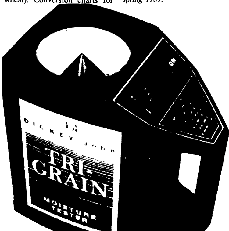
This portable grain moisture tester from Dickey-john features calibrations based on those developed for elevator and commercial testers.
