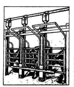
polyethylene feeders anywhere on straight runs of auger tubing. A simple ball valve is lifted by the central trip handle or power unit. Can be set to feed 11/4 to 10 lbs. of feed.
