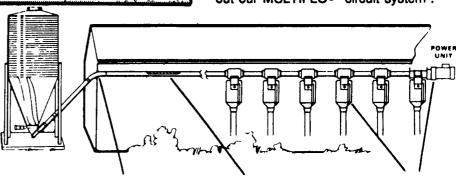
The coreless suge: moves feed around corners with no gears or wheels like other systems have. Ours is a study in simplicity!
