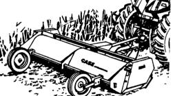
Use a Case International shredder to fine-shread heavy, tough cotton, com or sorghum stalks to speed decomposition, ease your tillage, planting and cultivating work. They're also useful for clipping pastures, shredding weeds, tall grass, or brush. And they actually require less power to operate because knives are spiralmounted around the rotor. • 170" wide.
