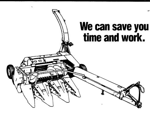
You get total performance when you harvest your crops with a Model 900 forage harvester. Total performance begins at the cutterhead The 12 knives of the 21-inch cutterhead give you uniformly cut high-quality forage Other features on the 900 include
