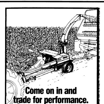
When it comes to harvesting, you can't beat the heavy-duty performance that's built into the New Holland Model 790 forage harvester. Performance starts at the cutterhead. The 19<sup>11</sup>/<sub>18</sub>-inch wide, 12-knife cutterhead delivers a fine uniform chop that's just right for most silage feeding operations. And an electric clutch gives instant response and positive control on the reversing gearbox. The Model 790 is available with either a 540 rpm or 1000 rpm PTO drive.
