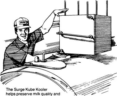
substantially reduces your milk cooling and water heating costs. And it does all this in less space — just a 22" cube
