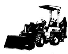
R400 Wheel Loader -Articulated Steering And Oscillating Frame, 38 H.P. Diesel Engine, One-Half Cubic Yard Bucket Capacity, 5 Forward-2 Reverse Speeds
