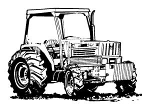
**M5950 DT** w/4 Post Rops and Canopy, 58 PTO H.P. 4 WD, 12 Synchronized Gears Forward, 4 Reverse Gears, Independent Rear PTO, Glow Plug Starting Aid, Power Steering, Front and Rear Differential Lock, Tilt Steering Wheel, Front Weight Set. 2 Remote Outlets
