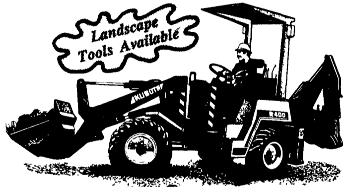
R400 Articulating Wheel Loader w/Backhoe
