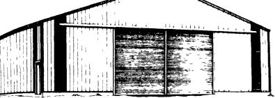
COMPLETE BUILDING - 40x60x12 INCLUDES PAINTED STEEL; 6x8 POSTS; 2x6 GIRTS; 2x6 PURLINS <u>BETWEEN</u> TRUSSES; 1 WALKDOOR & 1 18'x12' SPLIT SLIDING ENDWALL DOOR; CONTINUOUS FIBERGLAS RIDGE CAP. COMPLETE - ERECTED - INCLUDES TAX & DELIVERY - ONLY \$12,225.00 OTHER SIZES AVAILABLE
