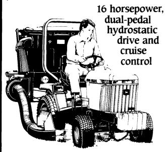
hydrostatic drive lets you change speed and direction on the go, in high or low ranges. That and standard cruise control keep your hands free for steering and other operations . keep vou productive with less fatigue Quik-Tatch feature lets you switch attachments in two nunutes. Liquidcooled 3-cylinder diesel. Optional frontwheel drive Call for a demonstration
