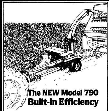
Holland, you get efficiency that's built in, not added on Standard features include: Flip-up feedroll, easy-adjust shearbar, electric clutch, hydraulic lift cylinder and two-speed blower. You also get a massive 12-knife cutterhead with hardened alloy knives with tungsten surfaces. And the knives are set at a steeper angle for smoother feeding and efficient chopping. Choose a 540 RPM or 1,000 RPM driveline. Stop in soon and see how the "790" can make your harvest faster and more efficient.
