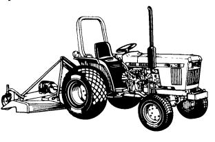
The John Deere 750 produces 20 hardworking horsepower from a fuel-efficient liquidcooled diesel engine. Optional front-wheel-drive is available if you need 4-wheel traction. Capacitymatched attachments are available to keep your tractor working all year long.
