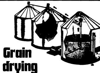
Shivvers automatic continuous flow grain drying systems eliminate the over-drying often caused by slow stirring devices. The Shivvers' secret is the tapered sweep auger which rotates around the drying bin, removing even layers of
