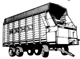
More speed Greater capacity And a price you can t beat anywhere. Good reasons to invest in a new Gehl 970 Series self-unloading forage box Look at all you get a 10-year warranty on sides. endgate stakes and platform new Even-Flow third beater wide 23-1/2-inch cross conveyor and two-speed worm gear drive. The 970 comes in five capacity sizes from 397 cu ft on the 14foot model up to 750 cu ft on the 18-foot model. See one today!
