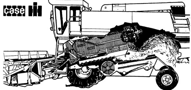
The one moving part in Axial-Flow's entire threshing/separating process is the single largediameter rotor. Nothing more. No cylinder, beaters or straw walkers. There's far less that can break or need maintenance. That's Axial-Flow combine simplicity.
