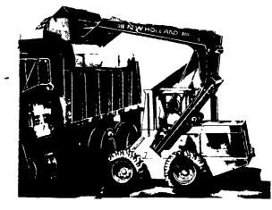
New Holland "Super Boom" loaders lift the payload forward as the boom rises. So you get more forward dump reach where you need it most. Extra dump reach means you can load the center of a tandem-axle dump truck.
