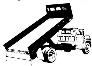
Rugged, all-steel 14" sides and 96" wide platforms. Heavy duty steel bulkhead with full width steel mesh window. Standard three-way express tailgate or optional double-acting tailgate with forward controls. More load space and hauling flexibility than a conventional dump body. These tough, field-proven units, teamed with job-matched Omaha Standard hoists, are total working units, superior to any on the market.
