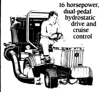
Unique dual-pedal hydrostatic drive lets you change speed and direction on the go, in high or low ranges. That and standard cruise control keep your hands free for steering and other operations keep vou productive with less fatigue Quik-Tatch feature lets you switch attachments in two minutes. Liquidcooled 3-cylinder diesel. Optional frontwheel drive Call for a demonstration.
