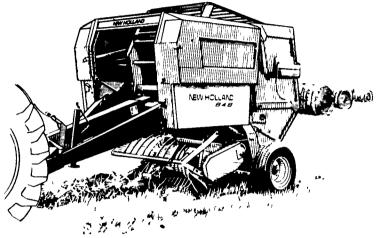
The Model 848 round baler is a high-capacity baler featuring a roll-floor design for a sure, fast core and increased bale density. The "848" makes bales four feet wide and up to four-and-a-half feet in diameter with a bale weight of 850 pounds. Choose one of three tying mechanisms: manual crank, hydraulic, or Bale Command<sup>™</sup> with Memory-Wrap<sup>™</sup>. Stop in and see the "848" today.
