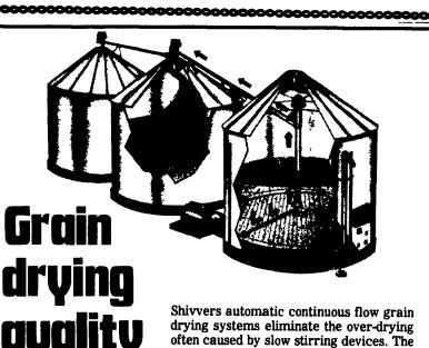
Shivvers automatic continuous flow grain drying systems eliminate the over-drying often caused by slow stirring devices. The Shivvers' secret is the tapered sweep
